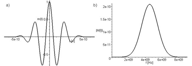
Figure 4: A typical Morlet a) waveform with a pulse width of 1 ns and center frequency of 4.5 GHz and b) its frequency spectrum
