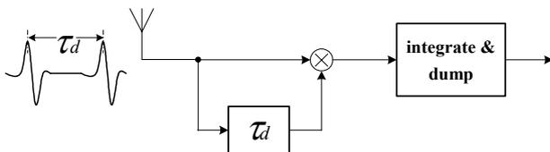
Figure 1: An autocorrelation receiver with a typical waveform
