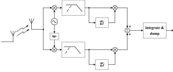
Figure 2: The proposed quadrature downconversion autocorrelation receiver
