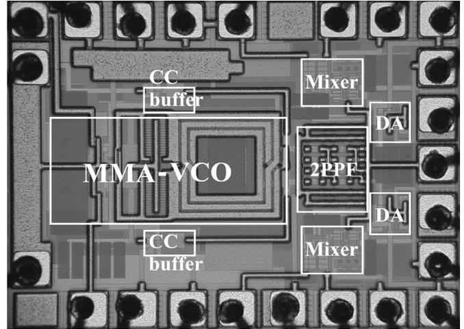
Fig. 6. Photomicrograph of the adaptive quadrature downconverter.
