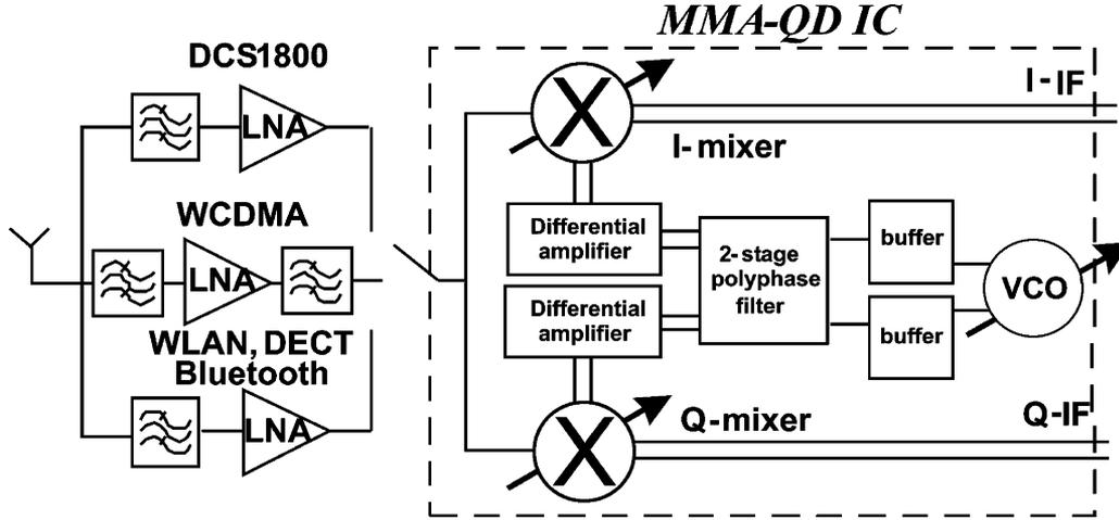
Fig. 2. Multistandard and adaptive receiver RF front-end.
