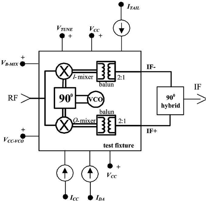
Fig. 8. Block diagram of the test setup.
