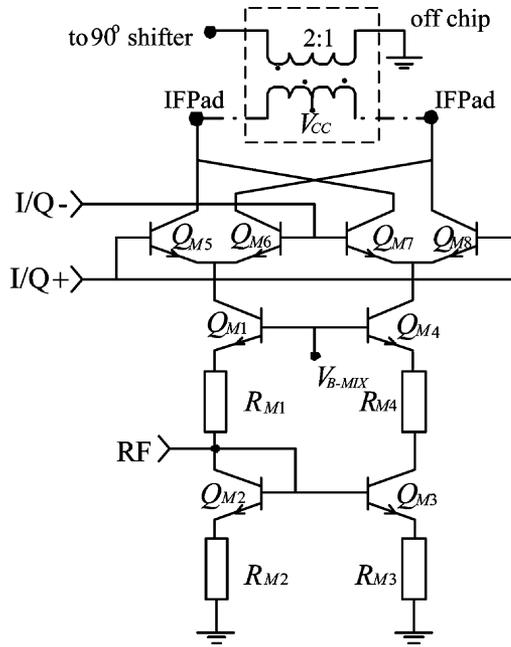
Fig. 5. Mixer with output transformer balun.
