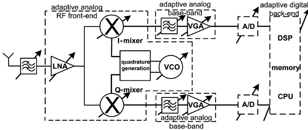
Fig. 1. Topology of an adaptive receiver.
