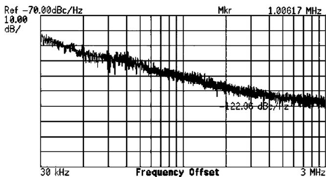
Fig. 10. Oscillator phase noise at 1 MHz offset from the 2.1 GHz carrier.
