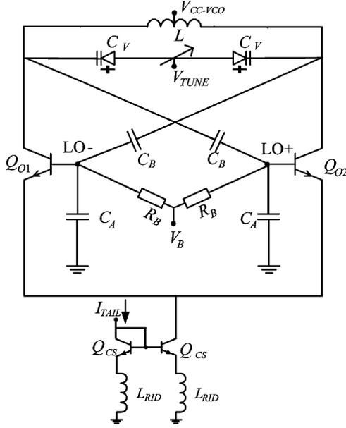
Fig. 3. Adaptive LC oscillator.
