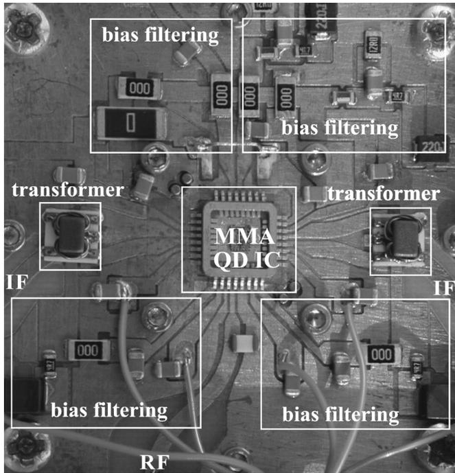
Fig. 7. Packaged multimode adaptive quadrature downconverter IC in the test fixture.
