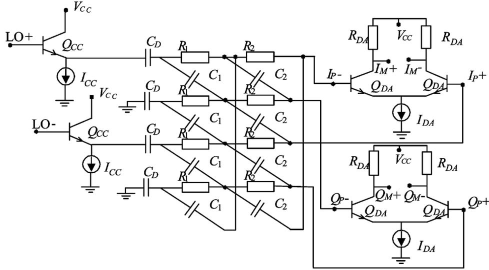
Fig. 4. Polyphase filter and buffer circuits.
