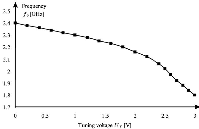
Fig. 9. Oscillator frequency-tuning curve for a 3 V tuning voltage.
