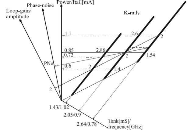
Fig. 6 *K-loop* diagram for the given parameters of the VCO.
