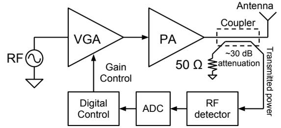
Fig. 1: Transmitted-power control loop
