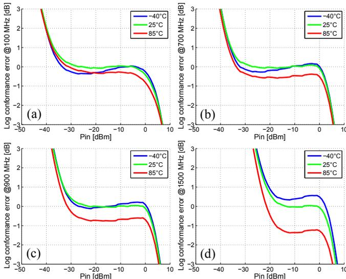
Fig. 10: Typical LCE for 100 (a), 700 (b), 900 (c) and 1500 MHz (d).
