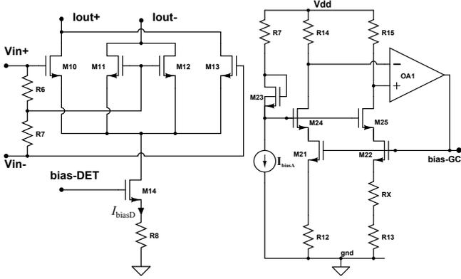
Fig. 5: Circuit of detector-cell (D) Fig. 6: Circuit of PTIM current generator.
