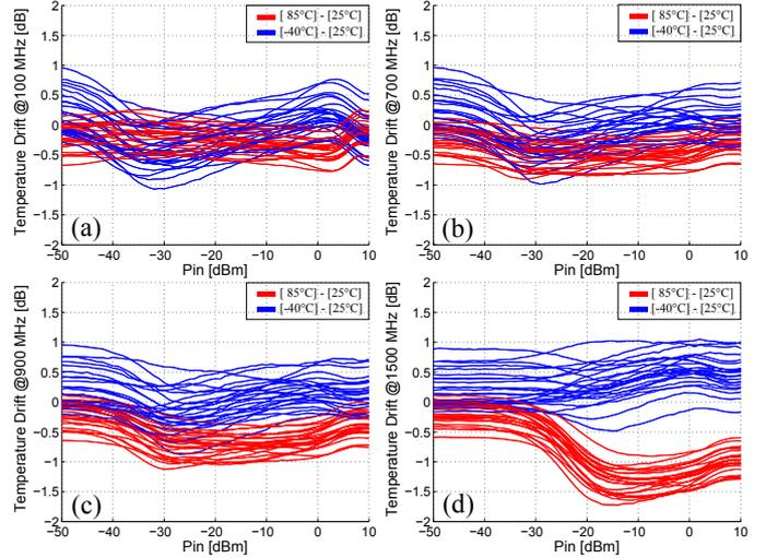
Fig. 11: Temperature Drift for 24 Samples at 100 (a), 700 (b), 900 (c) and 1500 MHz (d).
