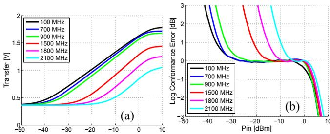
Fig. 9: Typical Detection Curves (a) and LCE (b) over frequency.
