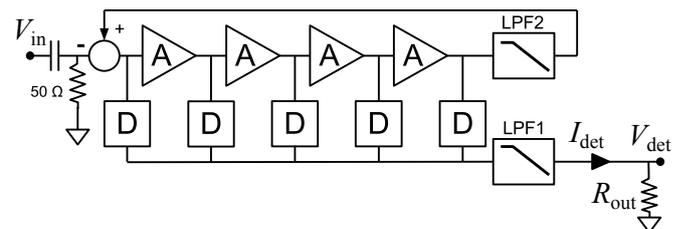
Fig. 2: Log-Amp Detector Core
