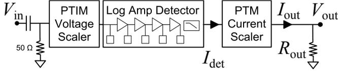
Fig. 3: Log-Amp Detector with temperature compensation
