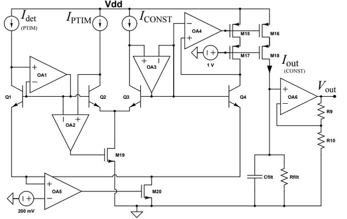
Fig. 8: Circuit of PTM current scaler and I-V converter.
