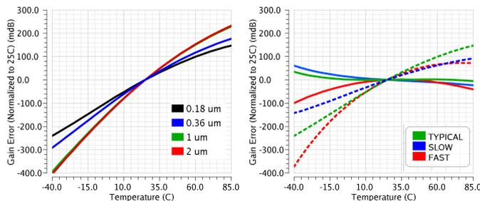
(a) Different L-sizes in bias generator, constant  $W/L$ ,  $L = 0.18 \mu\text{m}$  (dotted) cascodes in bias generator,  $L = 0.18 \mu\text{m}$  in gain cells and bias generator. (b) With- (solid) and without- (dotted) cascodes in bias generator,  $L = 0.18 \mu\text{m}$  in gain cells and bias generator.
