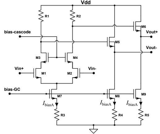
Fig. 4: Circuit of Gain-cell (A)
