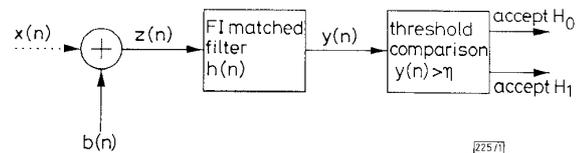
Fig. 1 Receiver structure
