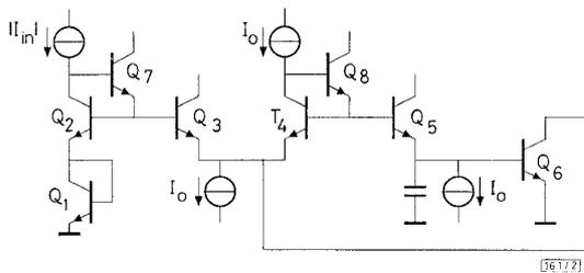
Fig. 2 Dynamic translinear RMSDC converter
