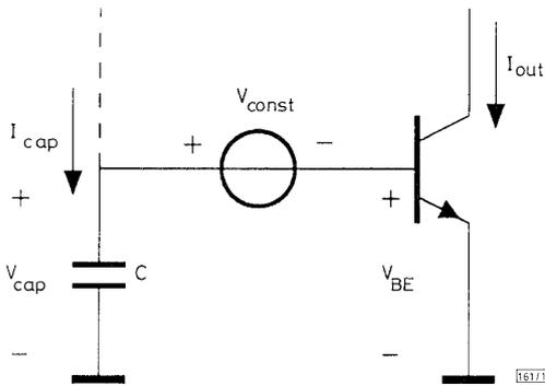
Fig. 1 Principle of dynamic translinear circuits
