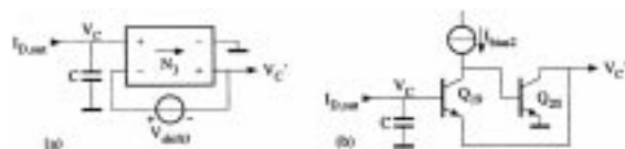
Fig. 7. Principle (a) and implementation (b) of the integrator/buffer.
