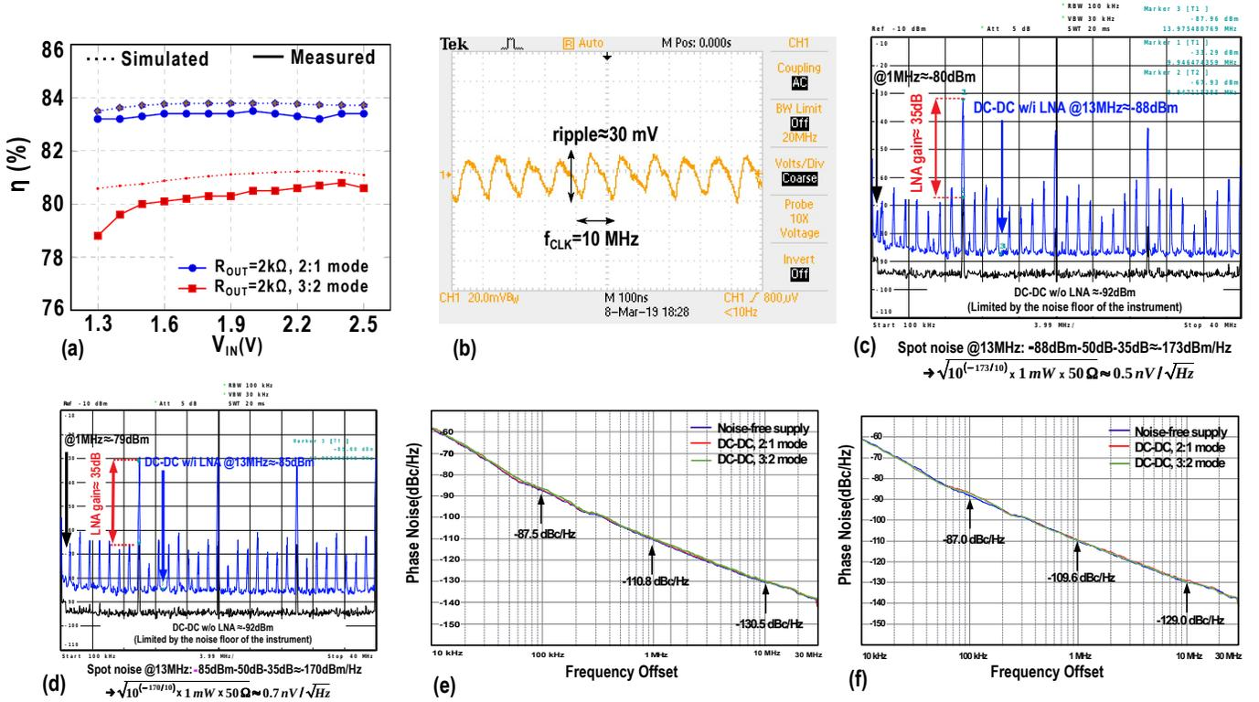
Fig. 15. (a) Measured power efficiency versus  $V_{IN}$ ; (b) output voltage of the DC-DC converter when directly connected to the oscillator; (c) spectrum of the output voltage of the DC-DC converter without (black line) and with (blue line) the use of an LNA in the 2:1 mode and (d) the 3:2 mode; (e) phase noise of the oscillator when powered by an ideal supply and the DC-DC converter in the 2:1 mode and 3:2 mode for  $f_0 = 5.5$  GHz and (f)  $f_0 = 4.9$  GHz.
