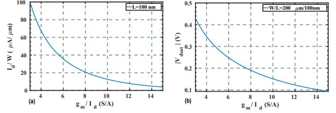
Fig. 2. (a) Current density and (b) overdrive voltage of the pass transistor for different  $g_m/I_D$  values.
