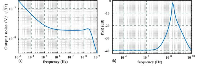
Fig. 5. (a) Simulated output noise and (b) PSR of the LDO using the component values reported in Table I.
