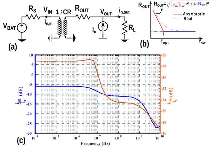
Fig. 8. (a) Equivalent model of a SC DC-DC converter with the noise current  $i_n$  used for the calculation of the transfer function; (b) its output resistance versus the switching frequency and (c) the simulated transfer functions from  $i_n$  to  $i_{n,in}$  and  $i_{n,out}$ .
