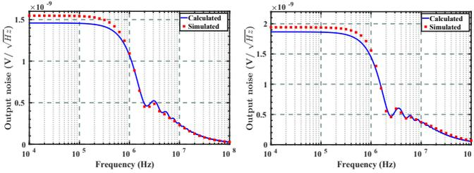
Fig. 10. Calculated (solid line) and simulated (dotted line) output noise of the DC-DC converter for the (a) 2:1 and (b) 3:2 configurations with  $C_{fly} = 1$  nF,  $C_{OUT} = 1$  nF,  $R_{on} = 30 \Omega$  and  $f_{SW} = 1.25$  MHz.
