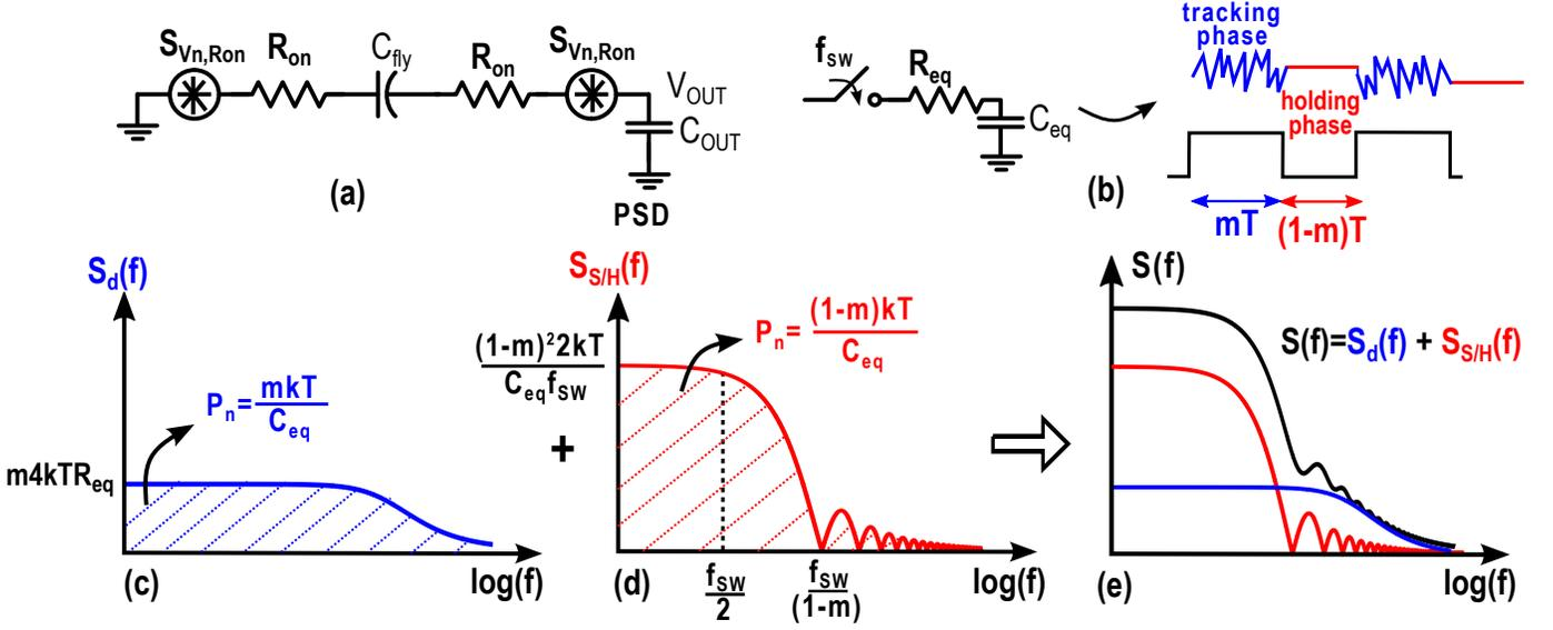
Fig. 9. (a) Equivalent circuit model for the DC-DC converter in the 2:1 mode (b) output noise waveform during the tracking and the holding phases (c) PSD of the resistor ( $R_{eq}$ ) shaped by the capacitor ( $C_{eq}$ ) during the tracking phase (d) PSD during to the holding phase and (e) a sketch of the total PSD (black line) due to the aliasing of the sampled noise.
