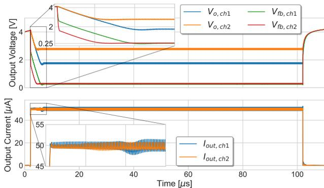
Fig. 8: Post-layout simulated output signals for a  $100\mu\text{s}$  (starting at  $t=2\mu\text{s}$ ) current pulse of  $50\mu\text{A}$  and  $R_{load,1}=30\text{k}\Omega$ ,  $R_{load,2}=50\text{k}\Omega$
