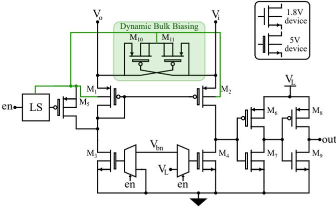
Fig. 4: Circuit implementation of the comparator.  $V_{bn}$  is the bias voltage for  $M_3$  &  $M_4$  when the comparator is enabled.
