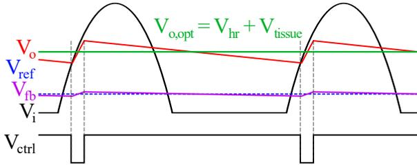
Fig. 2: Timing diagram of the proposed regulating rectifier circuit
