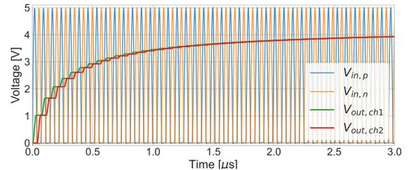
Fig. 7: Post-layout simulated start-up sequence with diode-connected rectifying switches.
