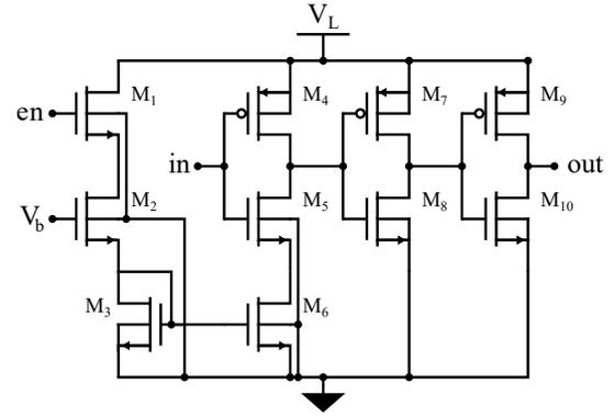
Fig. 5: Circuit implementation of the voltage-controlled delay line.
