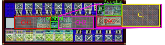
Fig. 6: Layout of the designed system with two channels
