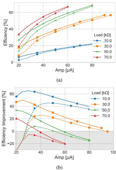
Fig. 9: (a) Simulated schematic (solid) and post-layout (dashed) efficiency of the proposed circuit as a function of output current for 4 load impedances, (b) Efficiency improvement of the proposed circuit with respect to a fixed  $5\text{V}$ -voltage supply
