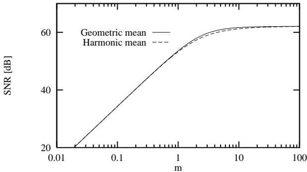
Figure 5: Signal-to-noise-ratio for different current splitters.
