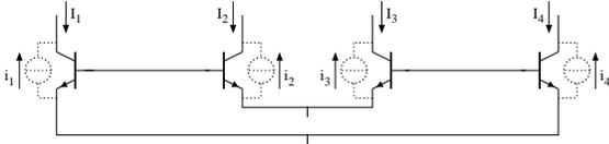
Figure 1: A second-order translinear loop in the presence of noise.
