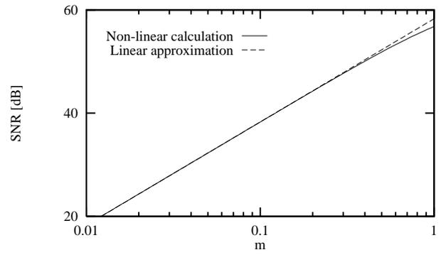
Figure 3: Signal-to-noise-ratio for a TL filter operated in class A.
