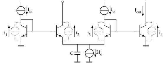
Figure 2: Noise in a translinear first-order low-pass filter.
