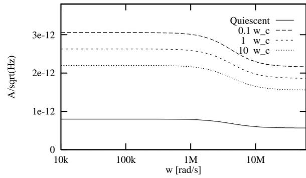
Figure 6: Influence of signal  $\times$  noise intermodulation on the noise spectrum.
