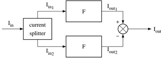
Figure 4: Set-up for class AB operation.
