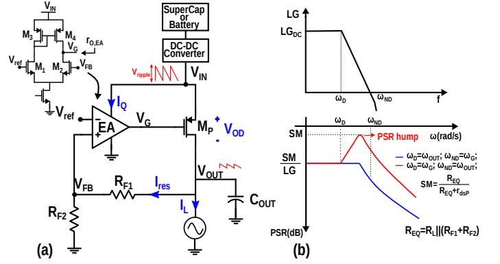
Fig. 1. (a) Block diagram of a typical LDO topology; (b) its PSR with (blue line) and without (red line) the use of an external capacitor.
