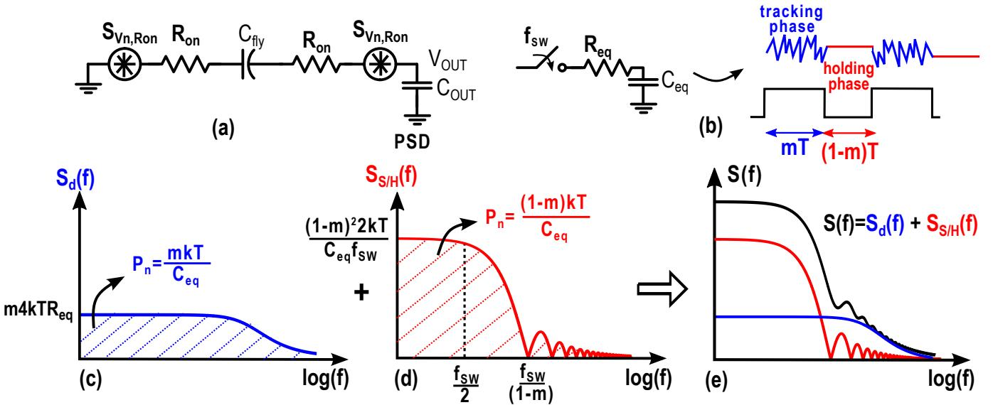
Fig. 9. (a) Equivalent circuit model for the DC-DC converter in the 2:1 mode (b) output noise waveform during the tracking and the holding phases (c) PSD of the resistor ( $R_{eq}$ ) shaped by the capacitor ( $C_{eq}$ ) during the tracking phase (d) PSD during the holding phase and (e) a sketch of the total PSD (black line) due to the aliasing of the sampled noise.
