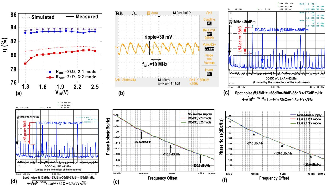
Fig. 15. (a) Measured power efficiency versus  $V_{IN}$ ; (b) output voltage of the DC-DC converter when directly connected to the oscillator; (c) spectrum of the output voltage of the DC-DC converter without (black line) and with (blue line) the use of an LNA in the 2:1 mode and (d) the 3:2 mode; (e) phase noise of the oscillator when powered by an ideal supply and the DC-DC converter in the 2:1 mode and 3:2 mode for  $f_0 = 5.5\text{ GHz}$  and (f)  $f_0 = 4.9\text{ GHz}$ .
