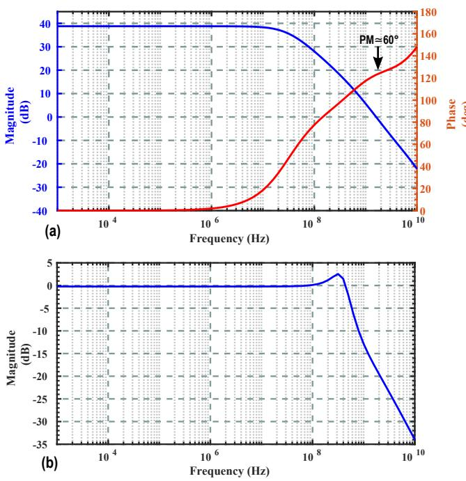
Fig. 4. (a) Open-loop transfer function of the LDO and (b) its transfer function from  $V_{ref}$  to  $V_{OUT}$  normalized to  $1/\beta$ .
