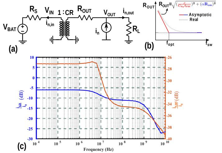
Fig. 8. (a) Equivalent model of a SC DC-DC converter with the noise current  $i_n$  used for the calculation of the transfer function; (b) its output resistance versus the switching frequency and (c) the simulated transfer functions from  $i_n$  to  $i_{n,in}$  and  $i_{n,out}$ .
