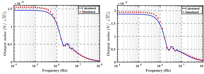
Fig. 10. Calculated (solid line) and simulated (dotted line) output noise of the DC-DC converter for the (a) 2:1 and (b) 3:2 configurations with  $C_{fly} = 1 \text{ nF}$ ,  $C_{OUT} = 1 \text{ nF}$ ,  $R_{on} = 30 \Omega$  and  $f_{SW} = 1.25 \text{ MHz}$ .
