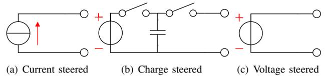
Fig. 2. Three fundamental system architectures
