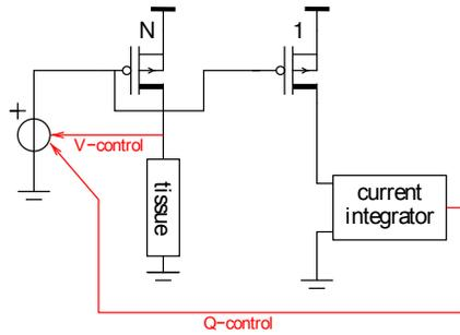
Fig. 3. Indirect current feedback with direct voltage feedback principle
