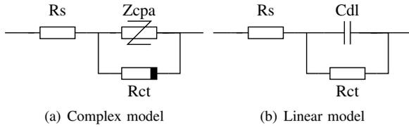
Fig. 1. Models for the Electrode-tissue interface
