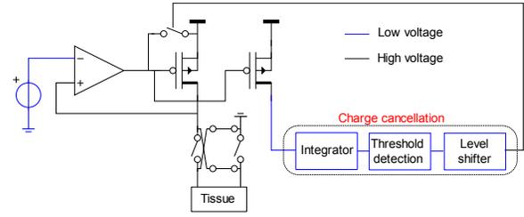
Fig. 4. Block diagram of the output stage employing double loop negative feedback
