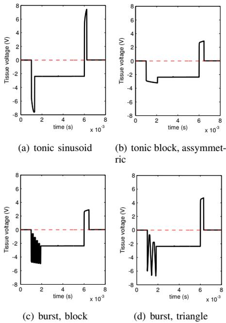
Fig. 5. Illustration of the flexible waveform possibilities
