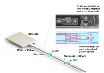
The layout of a microfabricated active optrode for neuroscientific research that allows for multi-site optogenetic neuromodulation and wide-bandwidth electrical recording. Credits: Ronaldo da Ponte, TU Delft. Not yet published.
